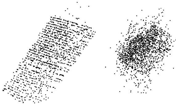
Figure 3. 3D reconstruction of book page without RANSAC. Left side shows the proposed method. Right side shows default matching.
