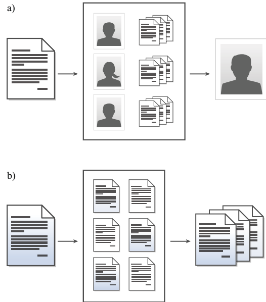
Figure 1. a) illustrates the task of writer identification. A new document is compared with all documents in the database and the result is the identity of the writer with the smallest difference. b) shows the task of writer retrieval. A new document is compared with all documents and a ranking of the similarity of the handwriting is generated.
