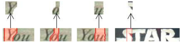
Figure 2. Multi-scale sliding windows with non-linear borders: from the left to the right, window widths are respectively h , \frac{h}{2} , \frac{3h}{4} and \frac{h}{2} .
