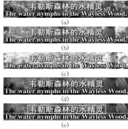
Figure 8. Example of text region refinement: (a)-(c) three text blocks in a series, (d) the result of MFI.
